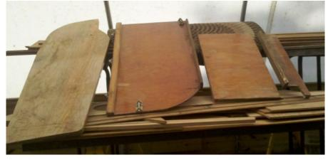
She is built of marine plywood and the covered with 2 layers of fiberglass cloth.
