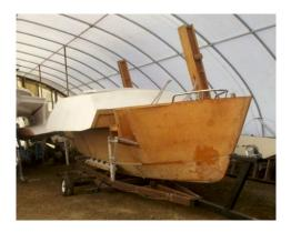
Draft 16 inches, 4ft 5" centerboard down, can run it right up on the beach. Folds up on the water to 8ft 3", so will fit in a slip 24ft long.
